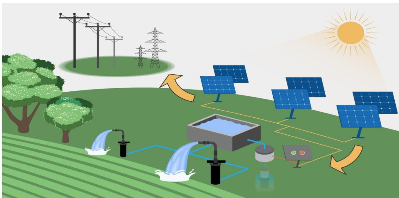
**Figure 4.** Solar irrigation system with net metering. Illustration by Aparna Nambiar.
