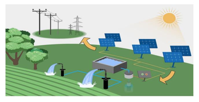
Figure 4. Solar irrigation system with net metering. Illustration by Aparna Nambiar.
